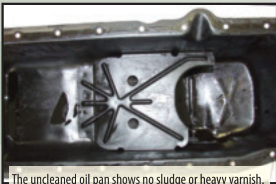
The uncleaned oil pan shows no sludge or heavy varnish.
